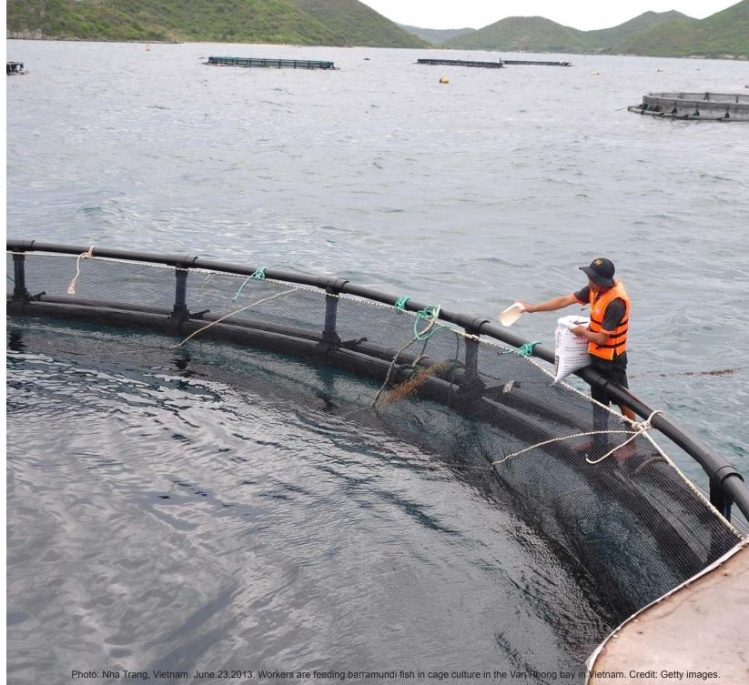
Industrial ocean fish farming facilities are exposed to severe marine conditions, including strong wind and wave activity from all directions, short and steep wave patterns, strong currents, seasonal anoxic (oxygen-lacking) conditions that can prevent operators from being able to access their cages, ranging in days to weeks.
